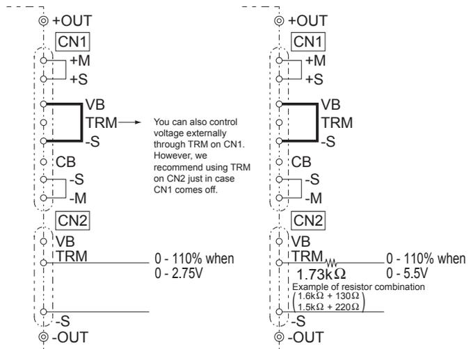
Fig.2.1 Wiring 1
