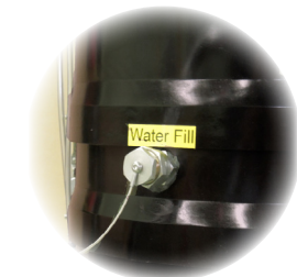
Water fill connection backflushes dispersion screen
