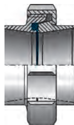
Complete ISO union S 2103 with Perbun sealing
