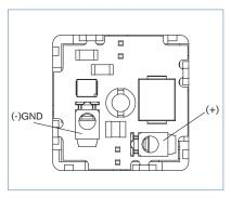
The high power electronics Type 2508HL increases the output of single solenoid valves. The high inrush power is generated by overexcitation. The adjustable pressure can be thus considerably extended. After switching the valve the electronic decreases to a small holding capacity. Also thereby power absorption and coil temperature in continuous operation can be much reduced. In holding operation the function is displayed by a yellow LED.
