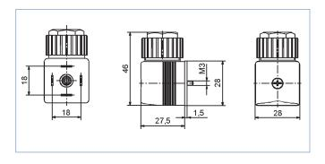
versions varistor, pole protection- and/or free wheeling diode (without LED) with black cover (polyamide)
