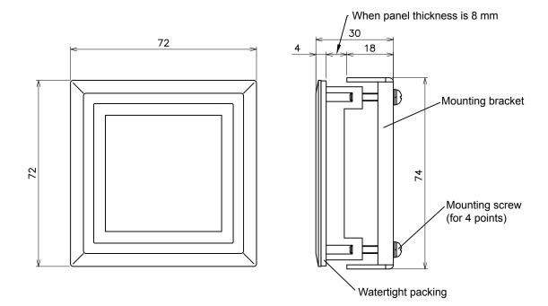
How to install PXF4 with the adapter
