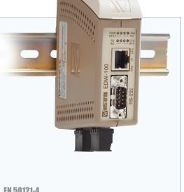
The EDW-100 is a serial to Ethernet converter designed to allow RS-232, RS-422 and RS-485 serial devices to communicate via TCP/IP Ethernet networks. DIP switches are used for configuration of RS-422/485 as well as for Ethernet port settings; the password protected web interface is used for all other settings. Diagnostic information can be accessed via a Telnet session with more basic information offered on LEDs.
