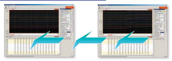
Use the supplied Logger Utility program to control real-time data recording from the PC. Scroll backward through the displayed trend graph window to view past waveforms even while recording.
