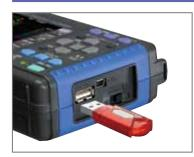
The LR8431-20 can record measurement data on a USB flash drive for easy transfer to a computer. In long-term measurement applications, it can also record to reliable Compact Flash cards for increased peace of mind.
