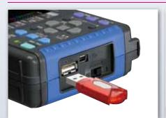
Real-time recording of up to 10ms/ sample data to USB or CF memory devices
