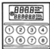
The heart of the MFA 10 summarizes functions that can be called up with 8 keys. It also displays the corresponding values on a two-line display panel and launches special functions. Monitors all sensor inputs and operates an error storage.
