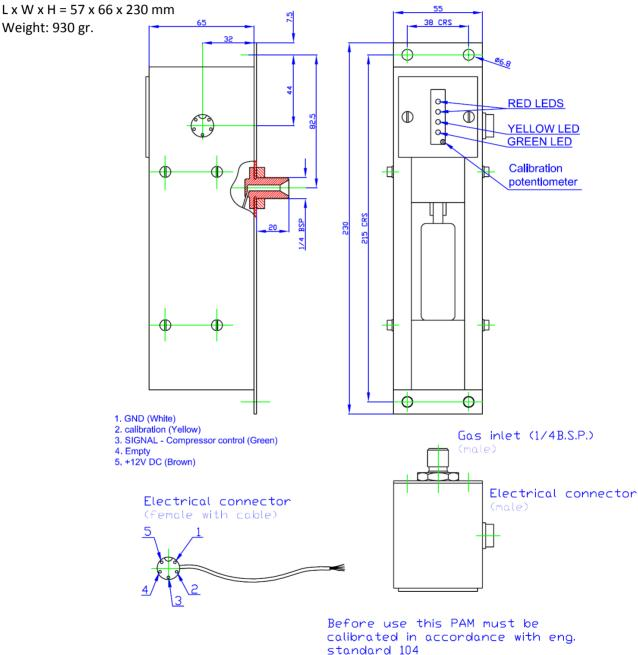
Picture 1: Scheme of PAM connected to high pressure generator for gas quality monitoring
