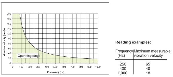
The operating range depends on the measuring range. The diagram shows that the rate of measurable vibration velocity falls as the frequency increases.
